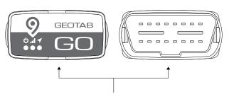
GPS antenna is located at the "bottom" of device.
