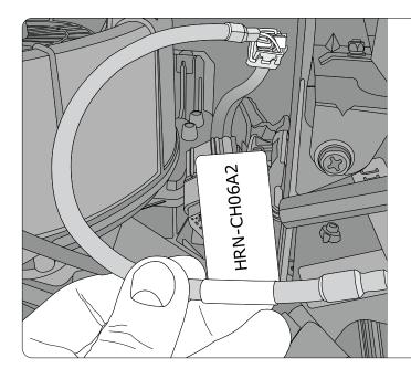
Step 4: Connect the HRN-CH06A2 to the factory 8-pin GPS connector.
