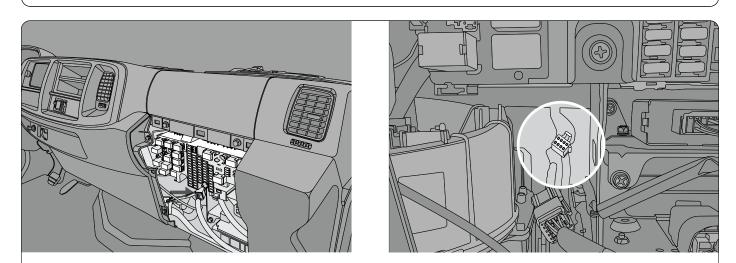
Step 2: Locate the blue 8-pin GPS connector at the back left of the fuse box.
