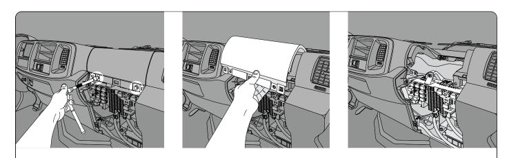
**Step 3:** Remove the upper passenger-side dash panel by removing the two 10 mm bolts.
