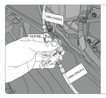
Step 5: Connect the HRN-CM24Y1 into the HRN-CH06A2. Be sure to connect both the J1939 and OBD-II 6-pin connections.
