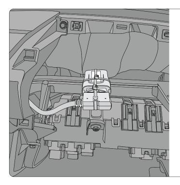
**Step 7:** Using zip ties, securely mount the GO device to the factory dash bracket above the fuse box.
