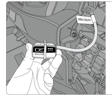
**Step 6:** Connect the GO device and secure it with the provided zip tie. Neatly run the GO device and cabling to the top dash to the left of the fuse box.
